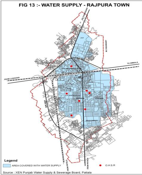
• As per data obtained from Executive Engineer Punjab Water Supply and Sewerage Division the total length of distribution line (mains and sub-mains) is 102 km and
